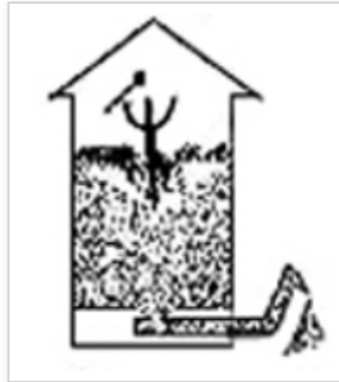
As unloading begins, bridged grain falls into the air space and the worker is instantly trapped.
