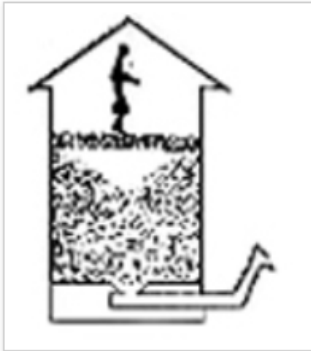
A dangerous situation created by a previous partial unloading of the bin.
